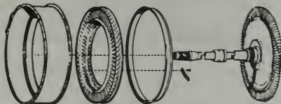
FIGURE 1-60. Turbine casing assembly.
